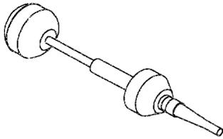
Unwired Removal Tool With Probe(s)
