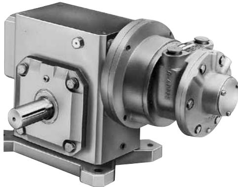
Max. allowable end thrust with 0 overhung load is 3552 lbs (1598,4 kg) at 30 rpm to 2154 lbs (969,3 kg) at 125 rpm. Max. overhung load on output shaft with 0 end thrust 2857 lbs (1285,7 kg).
