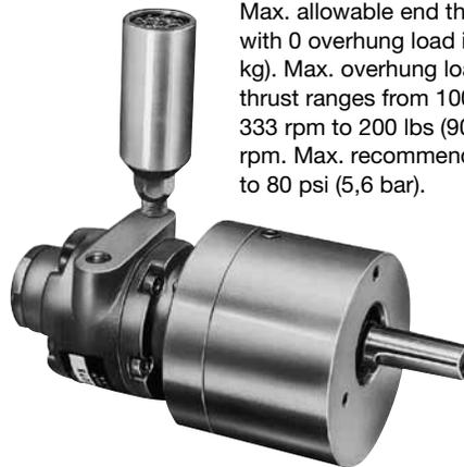
Max. allowable end thrust with 0 overhung load is 100 lbs (45,0 kg). Max. overhung load with 0 end thrust ranges from 100 lbs (45,0 kg) at 333 rpm to 200 lbs (90,0 kg) at 33,3 rpm. Max. recommended pressures to 80 psi (5,6 bar).
