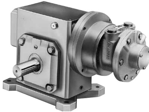
Max. allowable end thrust with 0 overhung load is 3552 lbs (1598,4 kg) at 30 rpm to 2154 lbs (969,3 kg) at 75 rpm. Max. overhung load on output shaft with 0 end thrust 2857 lbs (1285,7 kg).
