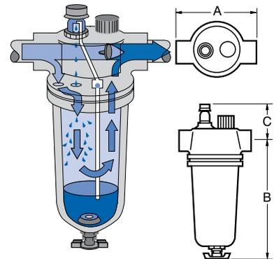
Mist lubricators provide uniform lubrication for the traditional lubricated style air motor. This results in reduced friction, extending the life of moving parts.
