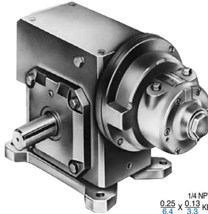
Max. allowable end thrust with 0 overhung load is 3545 lbs (1595,3 kg) at 10 rpm to 2134 lbs (960,3 kg) at 50 rpm. Max. overhung load on output shaft with 0 end thrust 1601 lbs (720,5 kg).
