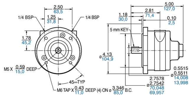
Delivers up to 0,56 kW ( $\frac{3}{4}$  HP). Speeds may be varied from 300 to 3,000 rpm. Max. recommended operating pressure 7 bar (100 psi).
