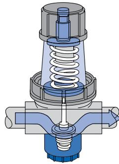
An air pressure regulator is necessary in most air motor applications to maintain a constant pressure regardless of the rise and fall of line pressure.
