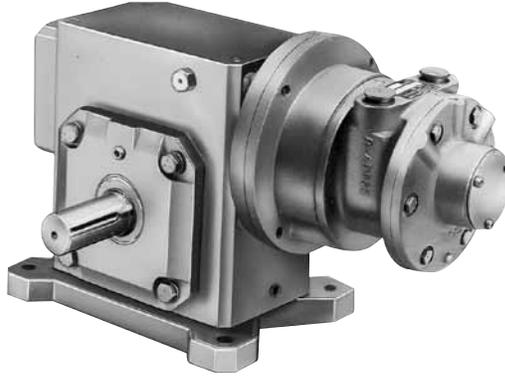
Max. allowable end thrust with 0 overhung load is 1640 lbs (738,0 kg) at 60 rpm to 923 lbs (415,4 kg) at 300 rpm. Max. overhung load on output shaft with 0 end thrust 1601 lbs (720,5 kg).
