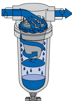
A filter helps ensure efficient operation by removing solid and liquid contaminants before they enter the air motor.
