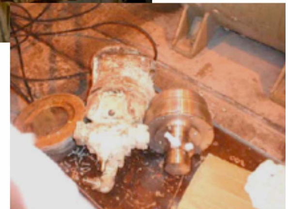
In comparison to DEPRAG: Low quality motor after operation
