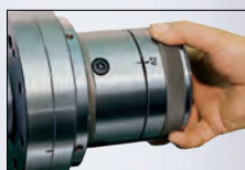
Hollow-center clamping with steel collet to DIN 6343
