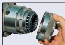
Clamping with collet and longitudinal workstop
